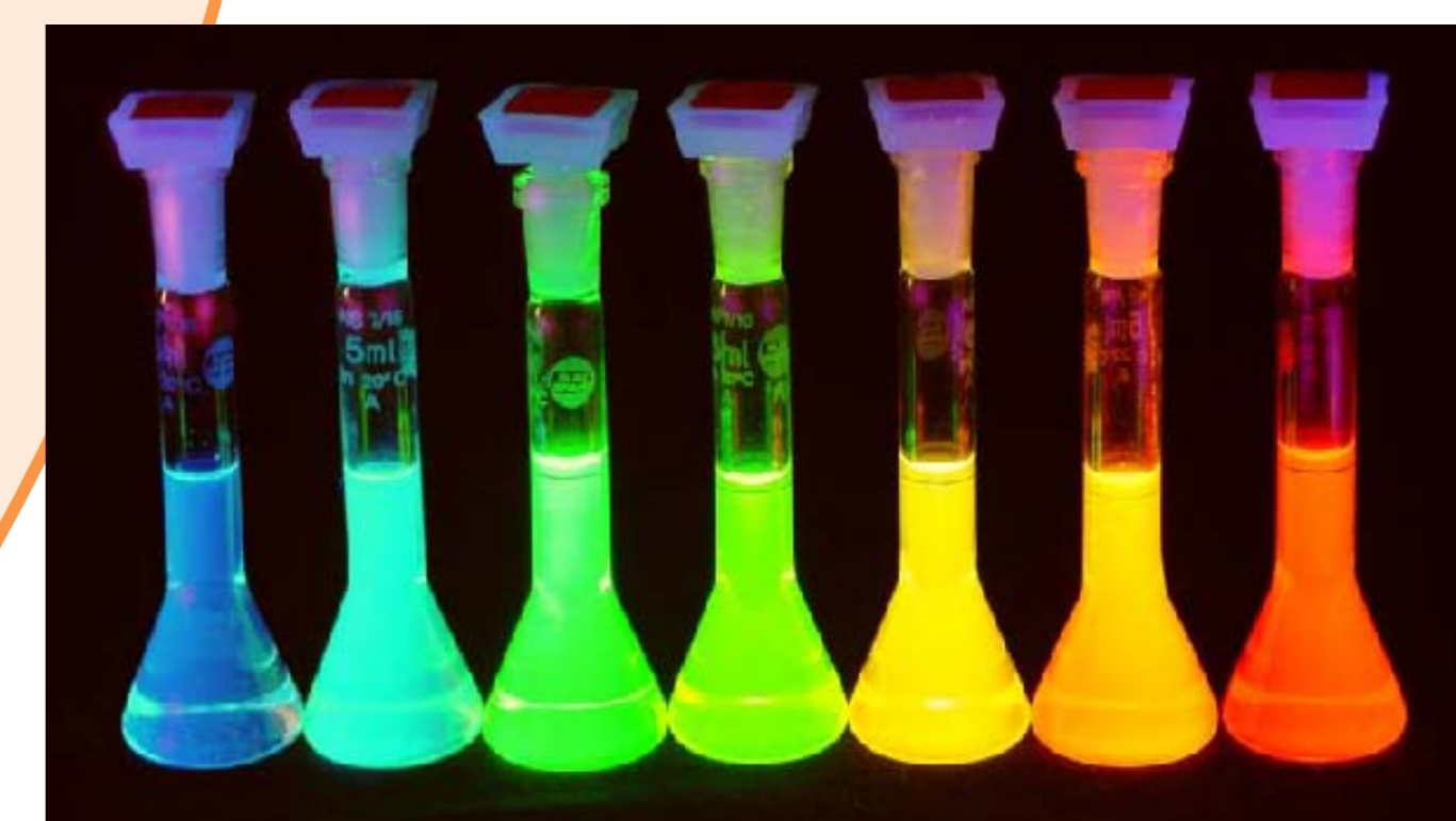
Fluorescent Q-dots emitting different colors upon irradiation with UV light
